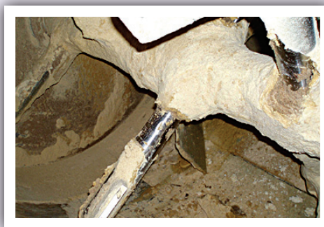
Figure 2: build-up of caking inside mixer
