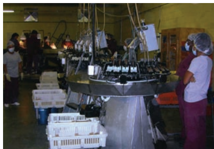
Interior view of the chick processing room showing feather sexing in progress (background) and beak treatment using Nova-Tech™ installations (foreground) at Brickland Hatchery.
