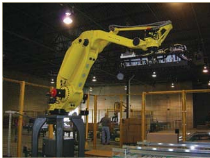
End-of-arm tool developed by Smart Motion Robotics to lift and transfer packed egg cases.
