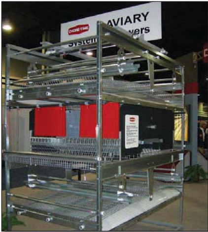
Chore-Time aviary module showing perching area, communal nest and feeding on vertically arranged tiers.
