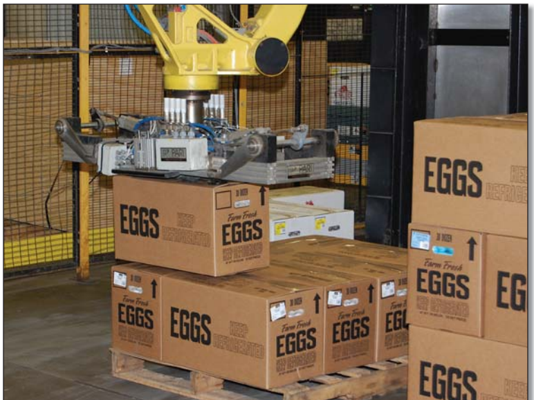
A robot is used on one packing line to stack off cases onto shipping pallets.
