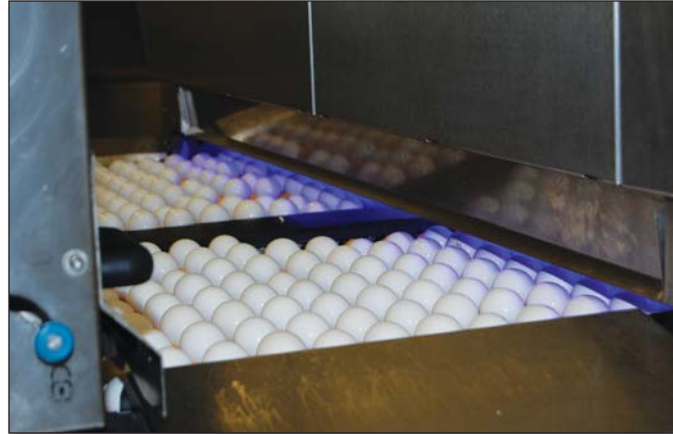
The Hyde County egg packing plant can clean, grade, pack and chill around 1,000 cases of shell eggs per hour.
