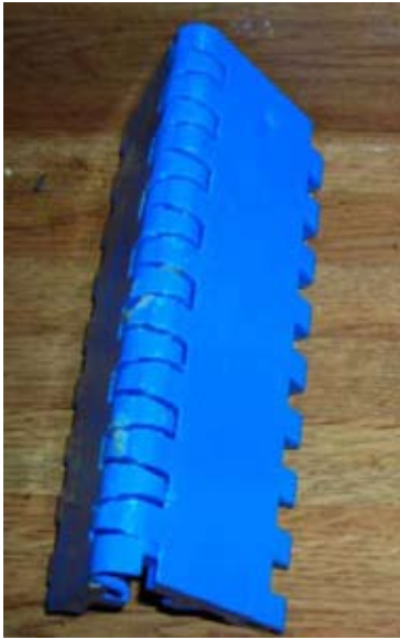
Plate 4 Meat residues remaining in hinges after cleaning/disinfection
