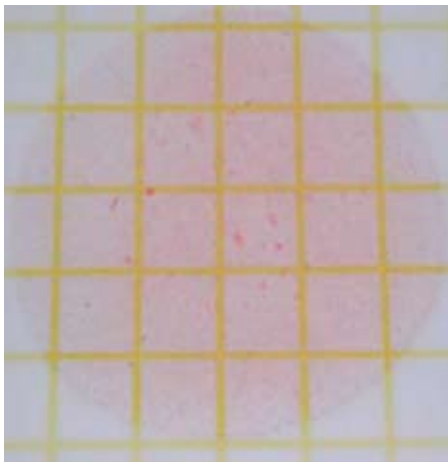
Plate 5 Petrifilm plate of bacterial count on hinge after cleaning/disinfection
