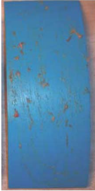
Plate 1 Sausage applied to PosiClean Material
