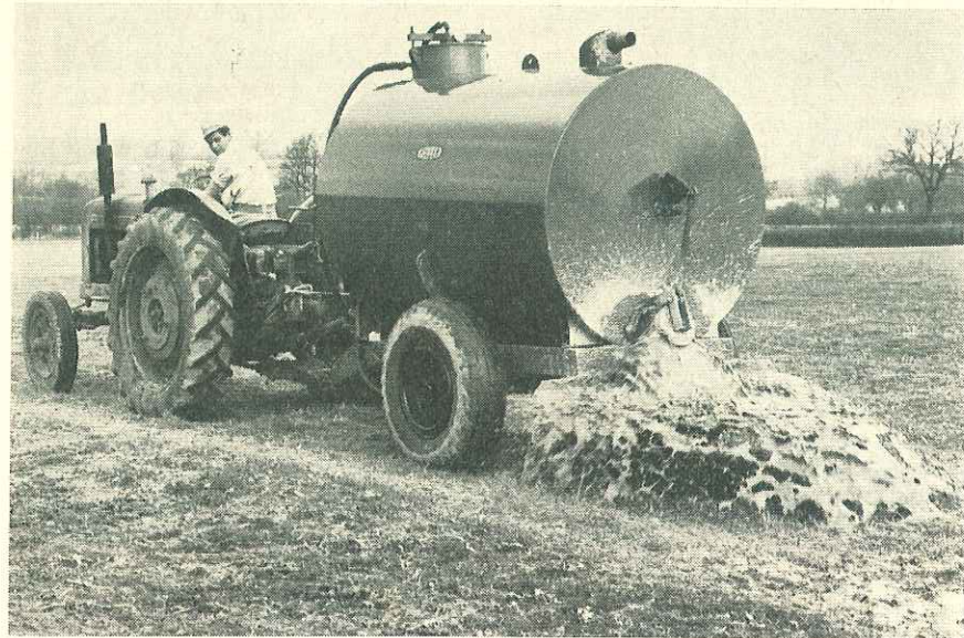
THE DRAWBACKS of tanker spreading include the need for somebody to be in attendance while the tanker is operating, and limited performance, which combine to make the labor requirement more than four times as much as pump-and-pipeline disposal. But a tanker is more maneuverable and can be shared by neighboring farmers.
