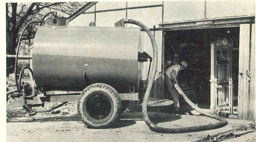
THERE IS A strong economic case for having the manure storage pit under the floor of the laying house. Droppings can then be scraped off the cage stacks to fall directly into the pit without any need for expensive mechanical conveyors. This indoor pit is being emptied with a vacuum tanker.
