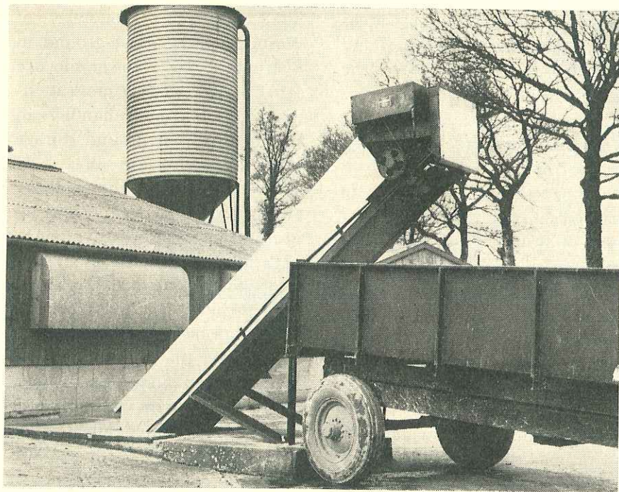
INSIDE THIS HOUSE, mechanical scrapers in under-floor channels convey the manure from the ends of the cage stacks to an elevator which loads a spreader parked underneath. This saves the cost of providing storage facilities but means that the manure has to be spread several times each week, whatever the weather and ground conditions.
