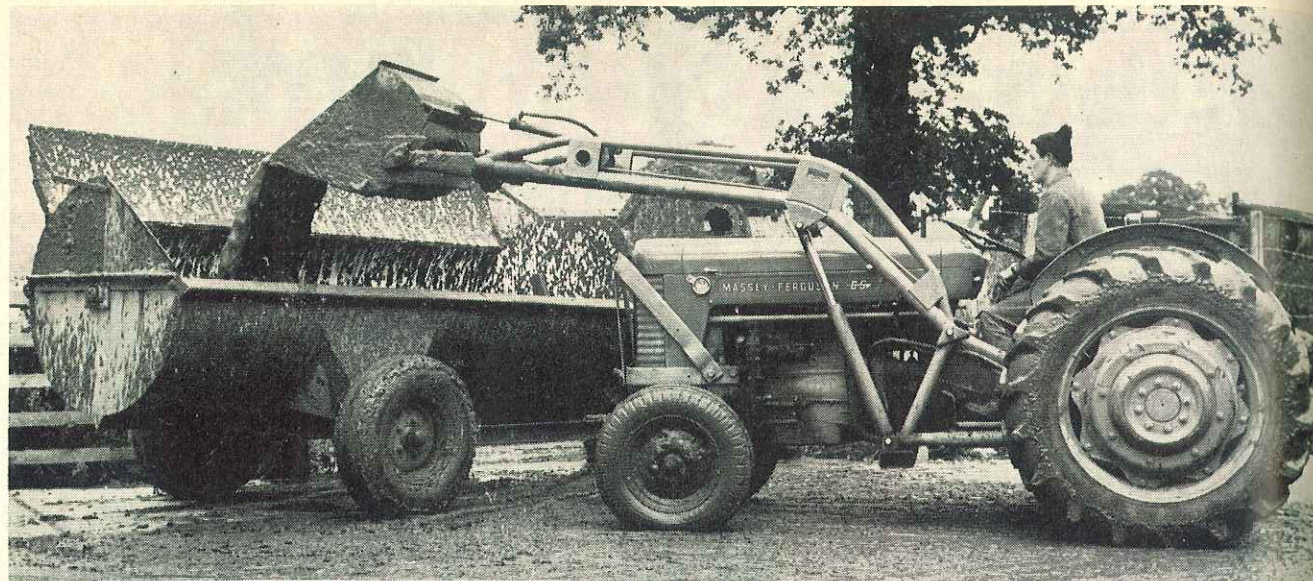
MANURE WHICH has been stored in a ground-level bunker is loaded into a rotary spreader by a tractor and scoop.
