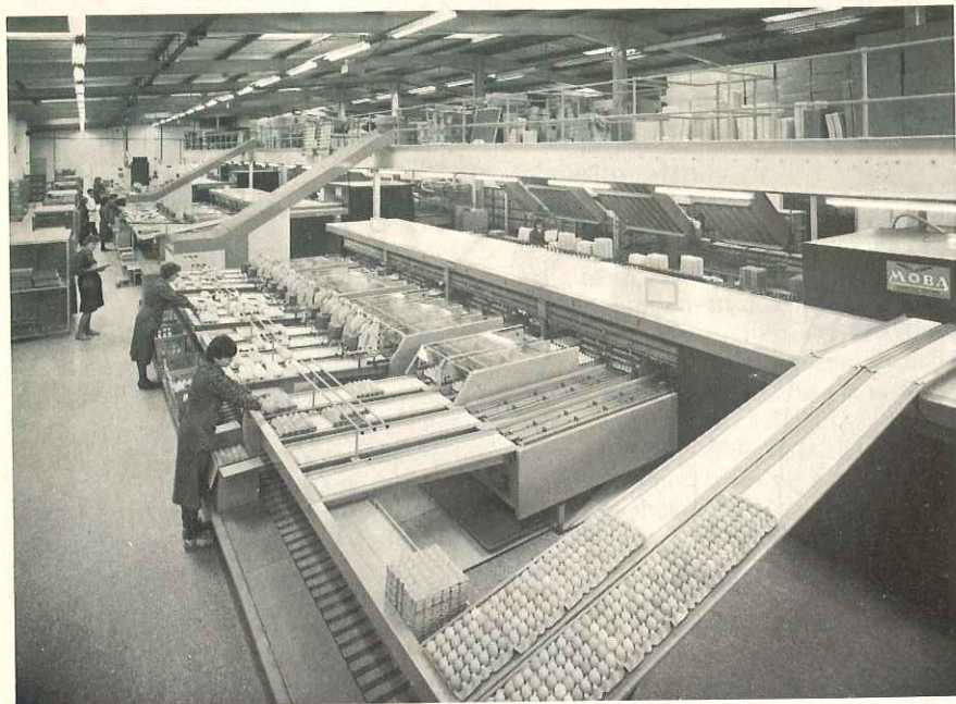
Some 25 000 cases of eggs can be graded and packed each week using three Moba 4000 machines.
