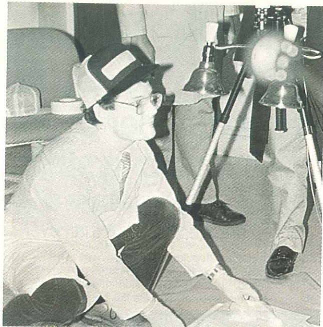
Programming a vision system is a demanding task. Engineers began programming their cut-up parts identification system by placing parts under the camera and capturing the resulting images into the computer's memory. From those images, they defined patterns the computer will use when examining a new image.
