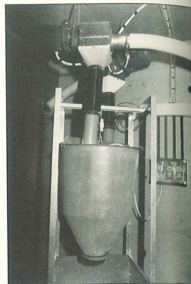
A combined feed weigher and blender which can service more than one house.
