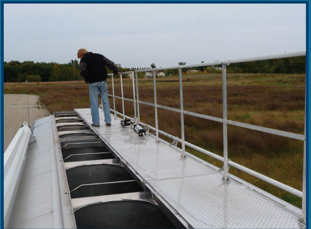
Walinga flip-up safety rails are on top of the trailer and offer fall protection for operators walking the aluminum catwalk.
