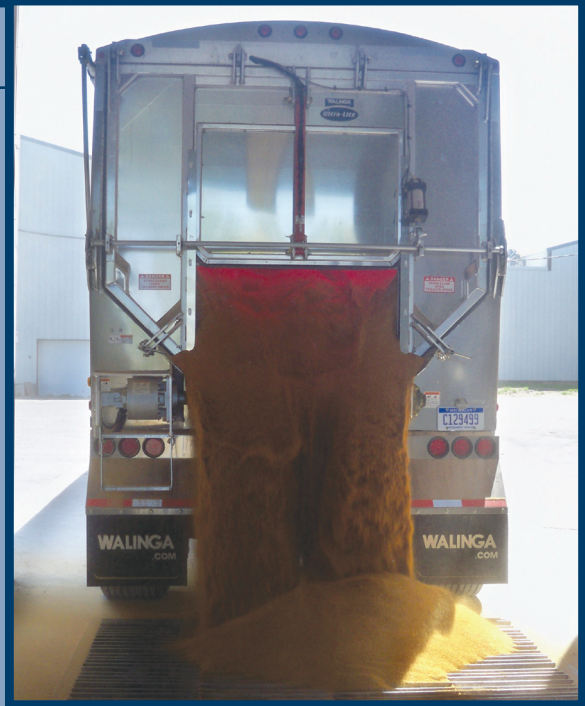
Brink Farms used to run trailers with walking floors, but replaced them with belt trailers to better suit its needs. The company now has two belt trailers.
