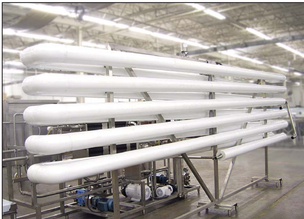
When designing a holding tube, it is important to consider the cinematic viscosities of all products to be processed as well as the speeds inside the tube.
