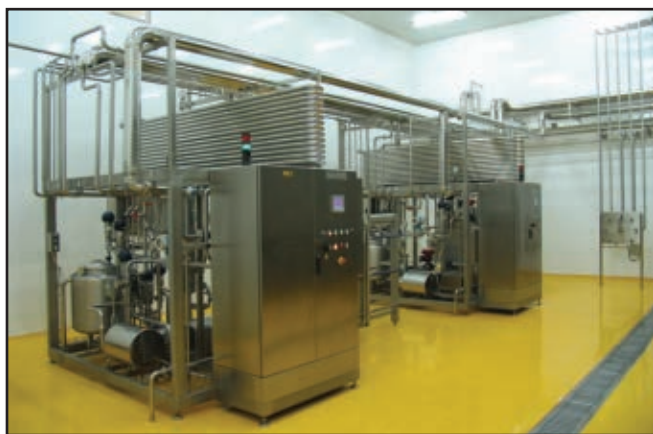
Sanovo pasteurization installations are available in two models with a capacity of up to 1,500 gallons/hour.
