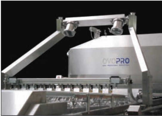
OvoPro 400S egg breaker separates liquid products with a capacity of up to 400 cph.
