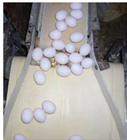
Incorrectly adjusted egg transfer areas can result in shell damage.
