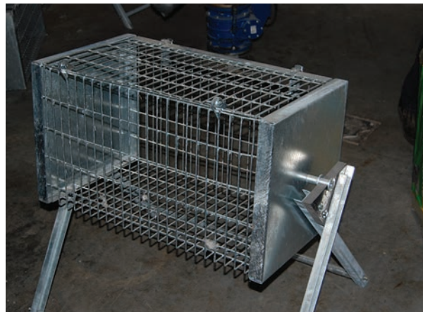
Alfalfa bales can be placed in a holder to give hens a distraction for pecking. It also rotates to make it harder for hens to camp out on top of it and quickly devour the bale. Terrence O'Keefe
