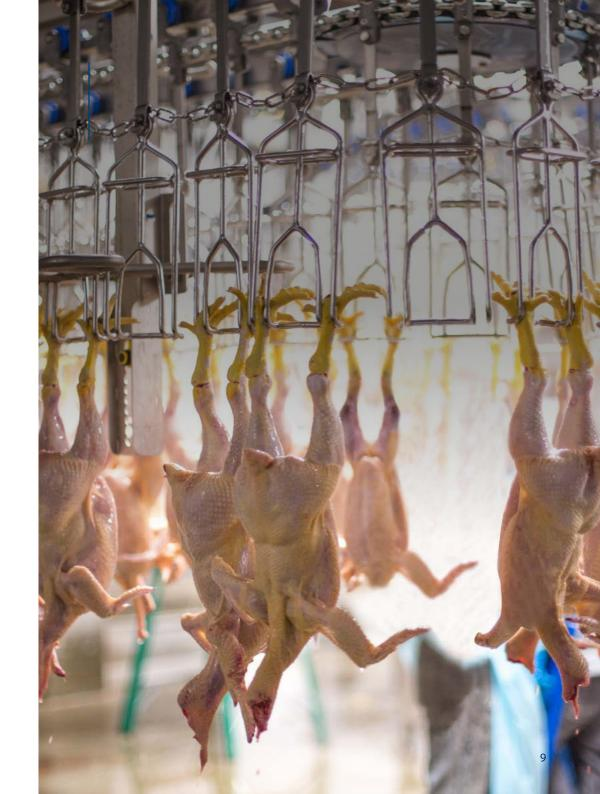
Empty shackles are also recorded. This allows processors to see any gaps in the hanging process, see if any birds might have dropped further down the line after the initial hanging, as well as provide some room between flocks, so the flock process and changeover can easily be identified.
