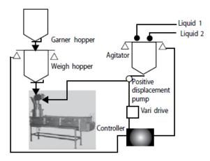
The advantage of this type of system is that the actual weight of the product is being monitored, so changes in density are accounted for. Also, calibration of this type of system is simple, since local scale companies can check the system calibration.
