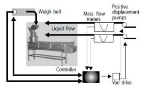
The preferred liquid meter in this case is a mass flow coriolis-type meter. This meter measures a shift in frequency and position of a tube that is proportional to the mass flowing through the tube. This in turn tells us the mass of product flowing through a tube in a specified period of time.
